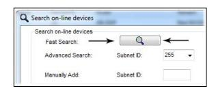
Fast search can't load all the Network Devices, it is only load part of the devices, it is only good for small project that contain around 10 devices, and to check the network communication with your PC.
